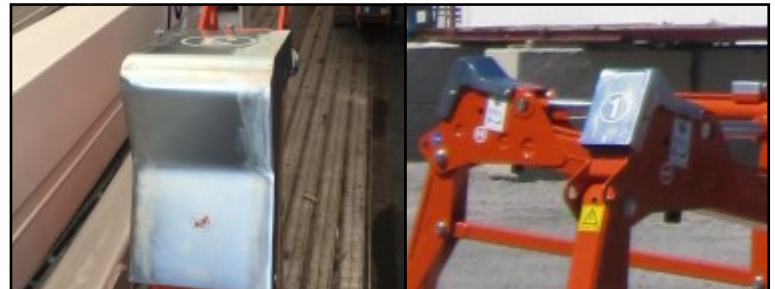
Stability switches HD galvanized covers
