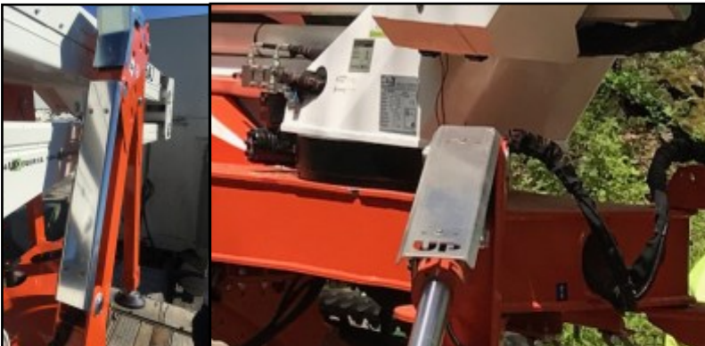
Outriggers thick aluminium plate protection
