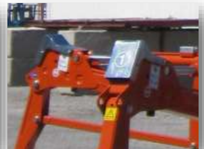
Stability switches HD galvanized covers
