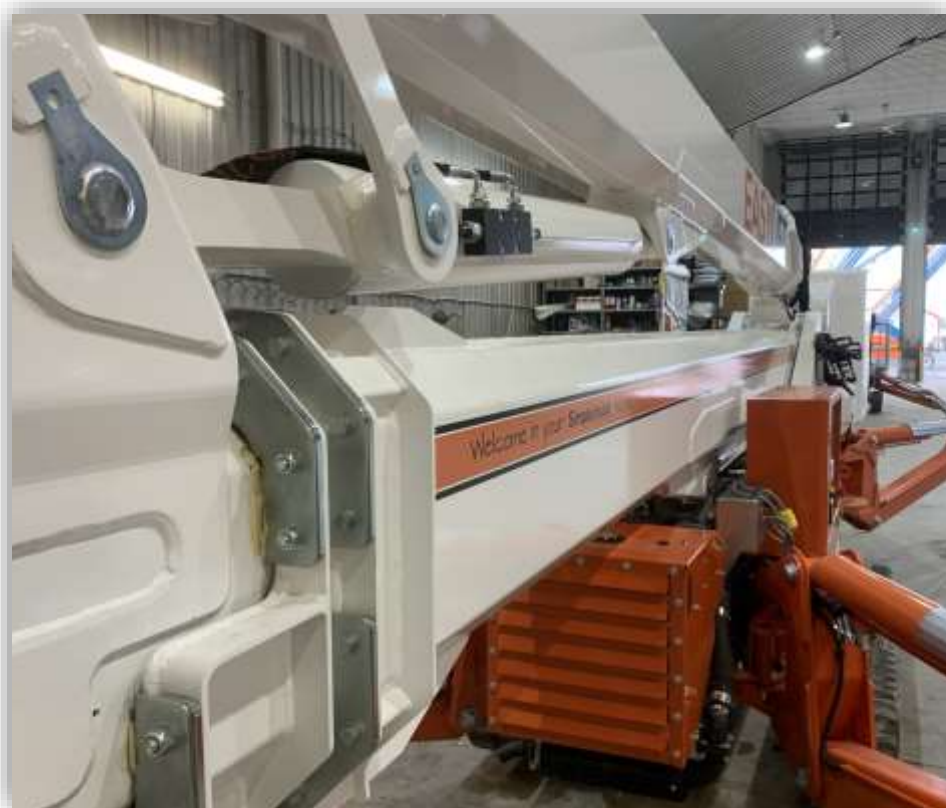
Super strong Octogonal shaped upper and lower booms
